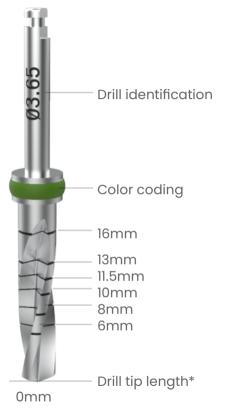
\* The length of the drill is measured from the tip to the middle of the depth marking
